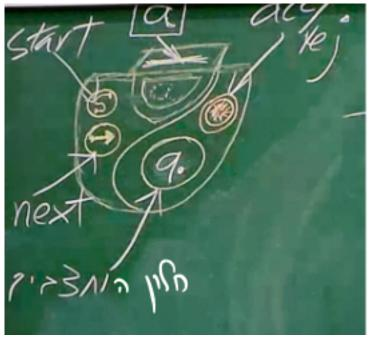
The automaton has a finite number of states, which are shown in this diagram at the window q. We press S to start, and the window shows  $q_0$ . When we press the right arrow, it uses the current letter from the input word to move to the next state  $q_1$ . Let us consider the input word aba.
